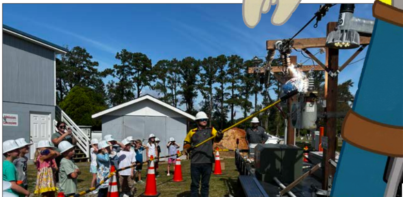
A Mylar balloon comes in contact with an energized line.
