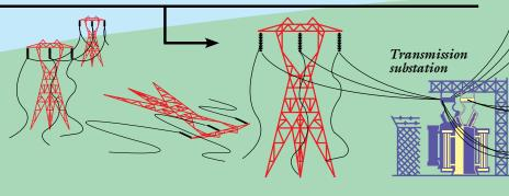
**Step 2.** A co-op may have several local distribution substations, each serving thousands of consumers. When a major outage occurs, the local distribution substations are checked first. A problem here could be caused by failure in the transmission system supplying the substation. If the problem can be corrected at the substation level, power may be restored to a large number of people.
