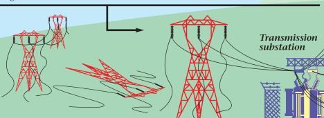
**Step 2.** A co-op may have several local distribution substations, each serving thousands of consumers. When a major outage occurs, the local distribution substations are checked first. A problem here could be caused by failure in the transmission system supplying the substation. If the problem can be corrected at the substation level, power may be restored to a large number of people.
